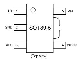
Output current can be adjusted above, or below the set value, by applying an external control signal to the 'ADJ' pin.
